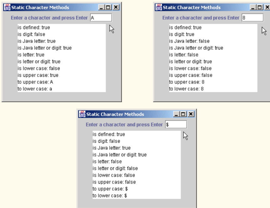
Fig. 10.17 static character testing methods and case conversion methods of class Character (part 3 of 3).
