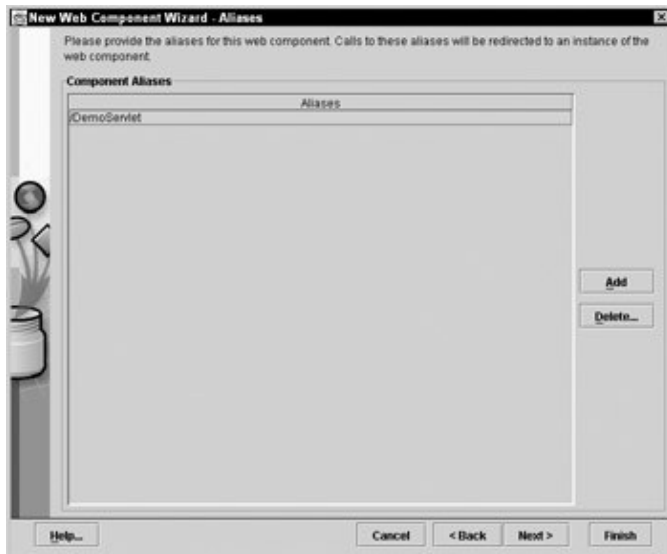
Figure A–27: Dialog in which you configure the aliases for the servlet class
