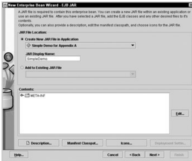
Figure A–5: The dialog that allows you to specify all the information needed for the EJB JAR file
