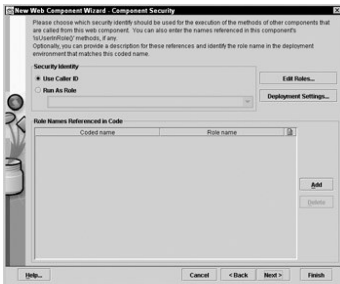
Figure A–28: Dialog in which you specify security–role information for each method in the servlet
