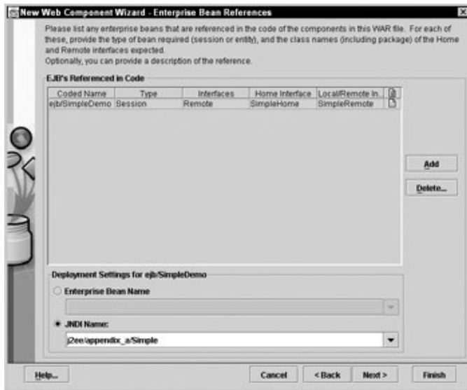
Figure A–31: Specification of the EJBs being referenced in the servlet code
