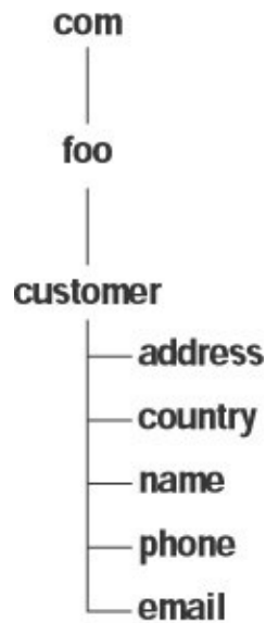
Figure 8–4: The arrangement of data for customer information in an LDAP directory tree
