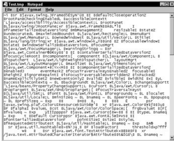
Figure 10–7: The extras in a serialized JFrame object
