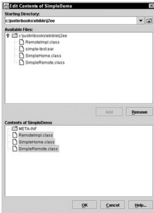
Figure A-6: Selecting the class files to be part of the EJB
