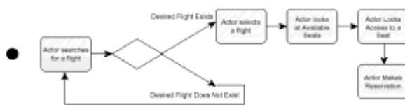
Figure 6.10: An activity diagram for the reservation system depicts the flow of work executed within the application as a whole.
