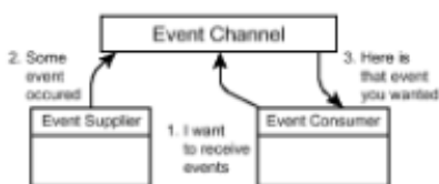
Figure 31.1: The CORBA Event Service functions with the aid of an event supplier, consumer, and channel.
