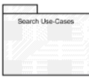
Figure 6.3: The use-case grouping relationship is modeled with the package symbol.
