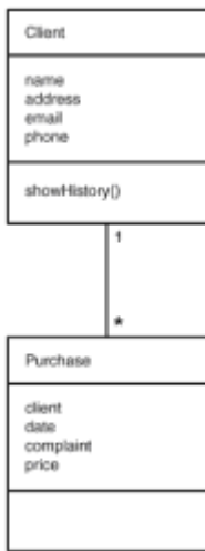
Figure 3.7: A class diagram can indicate associations.
