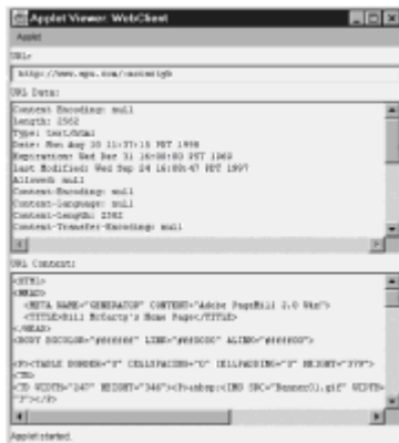
Figure 18.1: The WebClient applet displays the attributes and content of a Web document.
