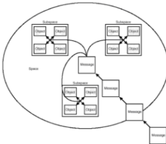
Figure 34.3: Message replication using Space technology.
