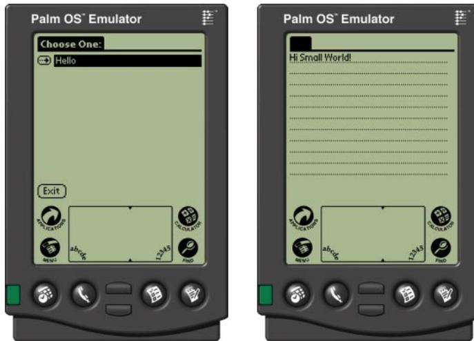
Figure 8.32 Running the HiSmallWorld MIDlet on the Palm OS device results in similar behavior as seen in the HiSmallWorld Spotlet developed with Jbed earlier. However, the user interface does have a little different look (see figure 8.26 for comparison).
