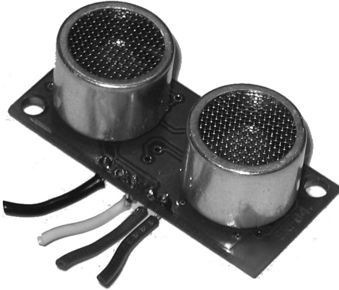
**Figure 4-15.** *The Devantech SRF04 Sonar Module*
