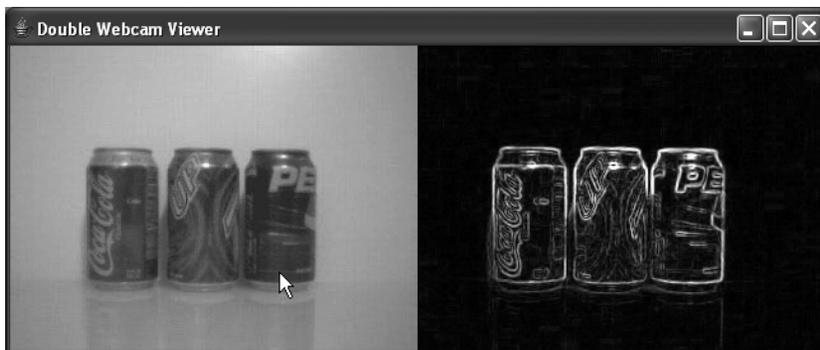
**Figure 6-23.** *The Sobel Gradient filter*
