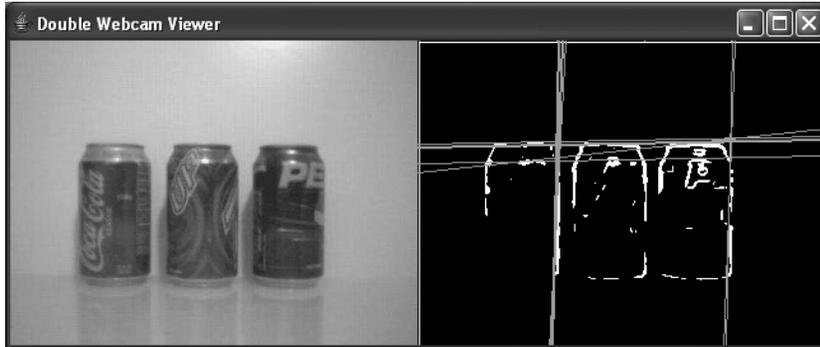
**Figure 6-24.** *The Hough transform of the three cans*
