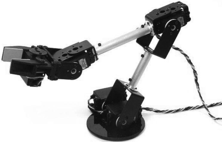
**Figure 3-11.** *The Lynxmotion Aluminum Arm*
