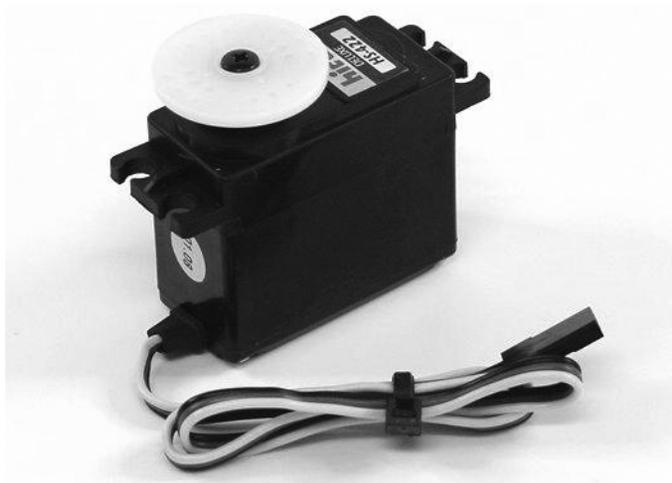
**Figure 3-1.** *The Hitec HS-422 Standard Servo (Lynxmotion Inc.)*
