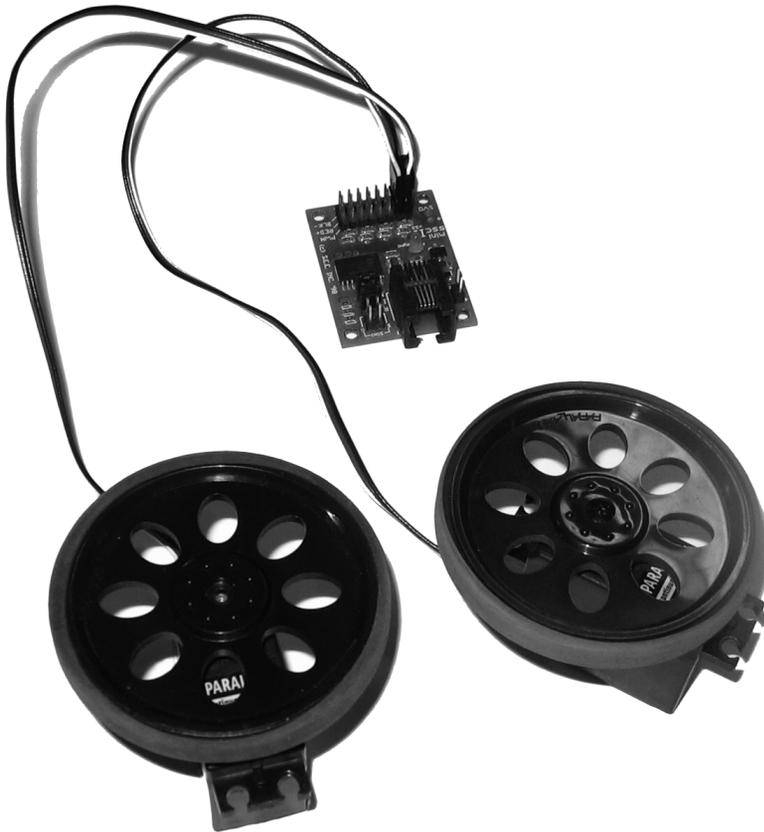
**Figure 3-2.** A servo controller and a servo with wheels
