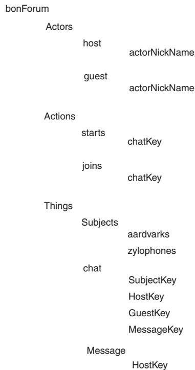
Figure 5.4 Designing bonForum XML using a tree diagram.
