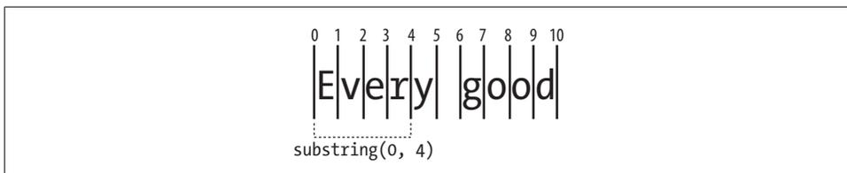
Figure 1-1. How `substring` end points are calculated
