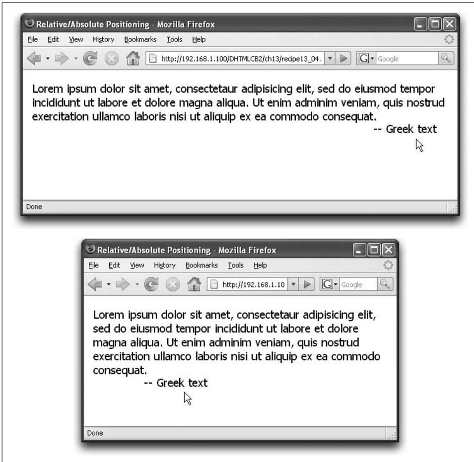
Figure 13-2. An absolute-positioned element inside a relative-positioned span element
