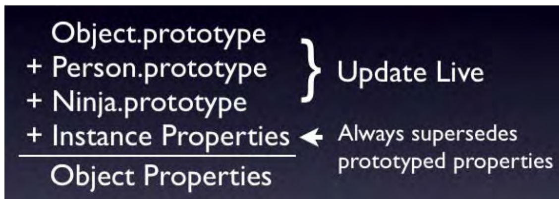
"Figure 5-1:" The order in which properties are bound to an instantiated object.
