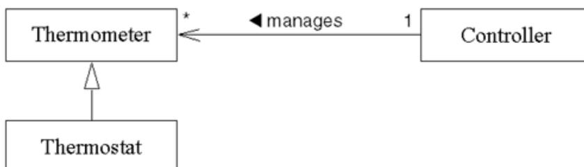
Each thermometer—and, by inheritance, each thermostat—has a mandatory association with exactly one controller. A controller manages any number of devices (possibly none). As indicated by the association arrow, we can navigate the association from the controller
