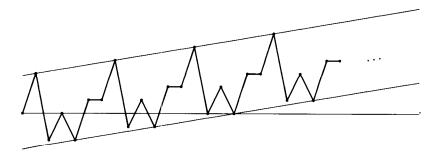
The entire graph can be contained between two lines of slope 1/m, as shown; we have m=6 in the illustration. In general these bounding lines touch the graph just once in each cycle of m points, since lines of slope 1/m hit points with integer coordinates only once per m units. The unique lower point of intersection is the only place in the cycle from which all partial sums will be positive, because every other point on the curve has an intersection point within m units to its right.
