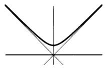
which has the lines y = x and y = -x as "asymptotes!' The curve approaches but never quite touches these asymptotes, when  $x \to \infty$ . Nowadays we use "asymptotic" in a broader sense to mean any approximate value that gets closer and closer to the truth, when some parameter approaches a limiting value. For us, asymptotics means "almost falling together!'
