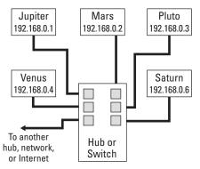
**Figure 5-3:** Five computers connected together through a hub or switch
