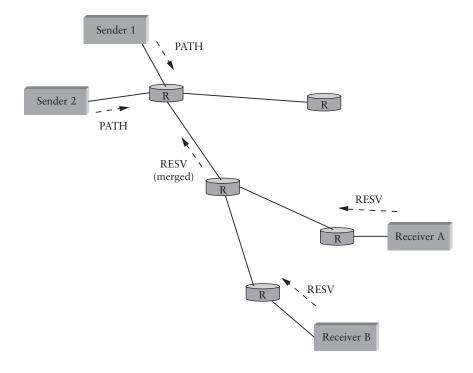
Figure 6.25 Making reservations on a multicast tree.
