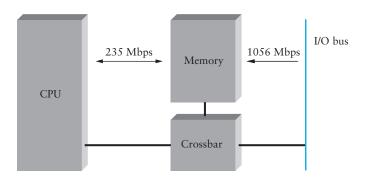
Figure 2.45 Memory bandwidth on a modern PC-class machine.
