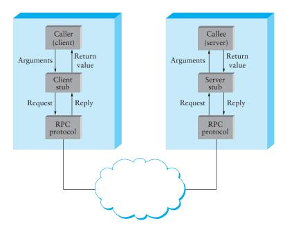
Figure 5.12 Complete RPC mechanism.
