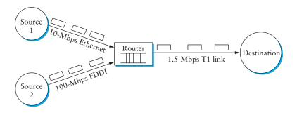
Figure 6.1 Congestion in a packet-switched network.
