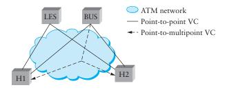
Figure 3.26 Servers and clients in an emulated LAN.
