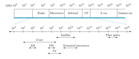
Figure 2.2 Electromagnetic spectrum.
