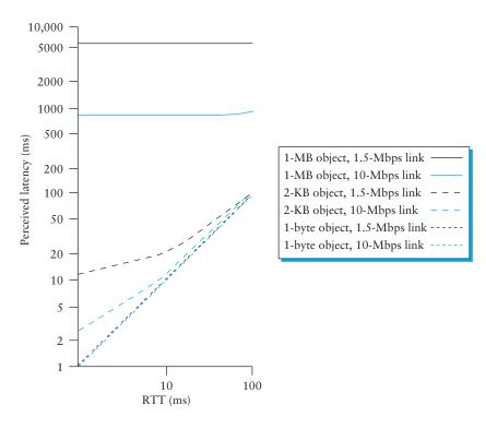
Figure 1.21 Perceived latency (response time) versus round-trip time for various object sizes and link speeds.
