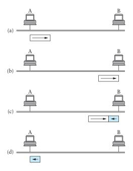
Figure 2.28 Worst-case scenario: (a) A sends a frame at time t; (b) A's frame arrives at B at time t + d; (c) B begins transmitting at time t + d and collides with A's frame; (d) B's runt (32-bit) frame arrives at A at time t + 2d.
