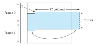
Figure 2.15 SONET frames out of phase.
