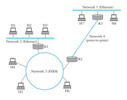
Figure 4.1 A simple internetwork. Hn = host; Rn = router.
