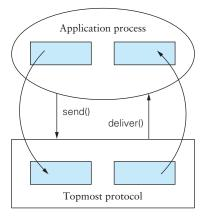
Figure 1.18 Copying incoming/outgoing messages between application buffer and network buffer.
