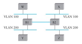
Figure 3.15 Two virtual LANs share a common backbone.
