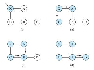
Figure 4.18 Flooding of link-state packets. (a) LSP arrives at node X; (b) X floods LSP to A and C; (c) A and C flood LSP to B (but not X); (d) flooding is complete.
