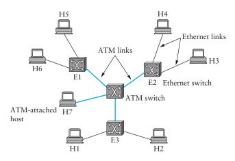
Figure 3.24 ATM used as a LAN backbone.
