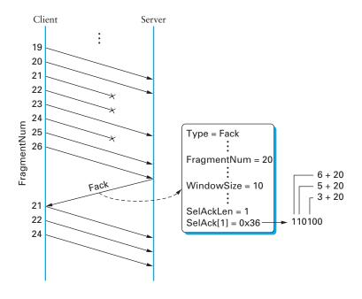
Figure 5.22 Fragmentation with selective acknowledgments.
