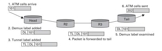
Figure 4.46 Forwarding ATM cells along a tunnel.
