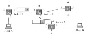
Figure 3.7 A packet makes its way through a virtual circuit network.
