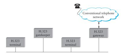
Figure 9.16 Devices in an H.323 network.
