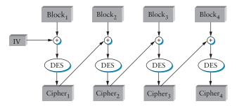
Figure 8.7 Cipher block chaining (CBC) for large messages.
