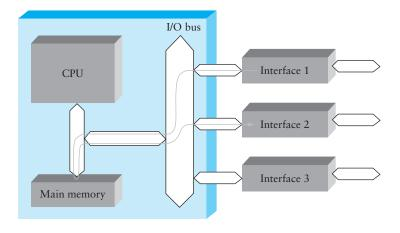
Figure 3.27 A workstation used as a packet switch.
