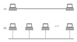
Figure 1.2 Direct links: (a) point-to-point; (b) multiple-access.
