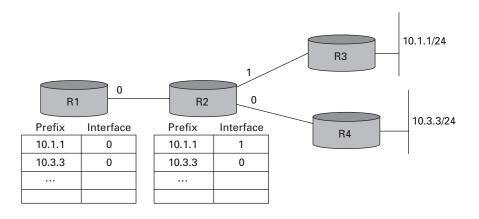
Figure 4.40 Routing tables in example network.
