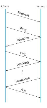
Figure 5.21 Typical DCE-RPC message exchange.
