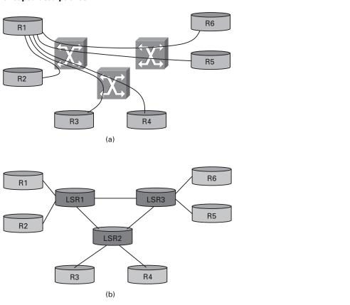
Figure 4.43 (a) Routers connect to each other using an "overlay" of virtual circuits. (b) Routers peer directly with LSRs.
