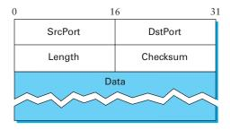
Figure 5.1 Format for UDP header.
