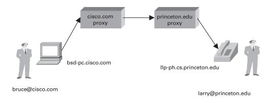
Figure 9.14 Establishing communication through SIP proxies.
