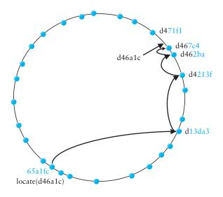
Figure 9.24 Objects are located by routing through the peer-to-peer overlay network.
