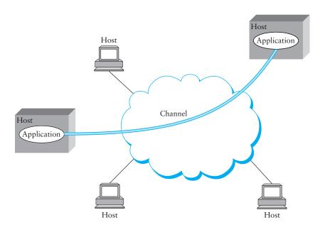
Figure 1.7 Processes communicating over an abstract channel.
