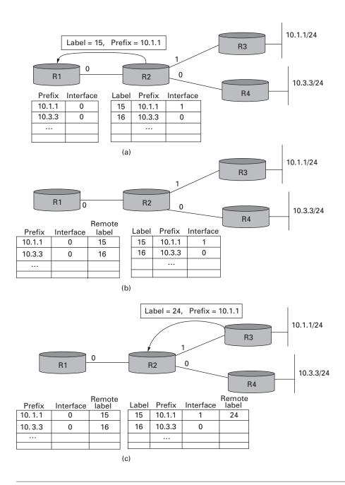
Figure 4.41 (a) R2 allocates labels and advertises bindings to R1. (b) R1 stores the received labels in a table. (c) R3 advertises another binding, and R2 stores the received label in a table.
