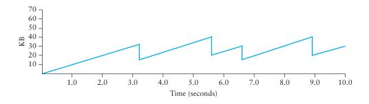
Figure 6.9 Typical TCP sawtooth pattern.
