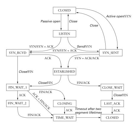
Figure 5.7 TCP state transition diagram.
