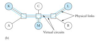
Figure 4.12 An example of virtual private networks: (a) two separate private networks; (b) two virtual private networks sharing common switches.
