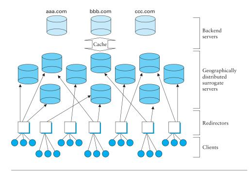
Figure 9.27 Components in a content distribution network (CDN).
