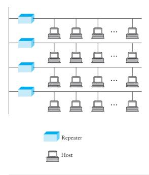
Figure 2.25 Ethernet repeater.
