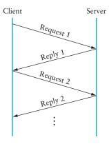
Figure 5.16 Timeline for CHAN when using implicit ACKs.
