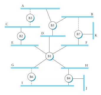
Figure 3.14 Spanning tree with some ports not selected.
