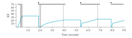
Figure 6.11 Behavior of TCP congestion control. Colored line = value of Congestion-Window over time; solid bullets at top of graph = timeouts; hash marks at top of graph = time when each packet is transmitted; vertical bars = time when a packet that was eventually retransmitted was first transmitted.
