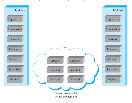
Figure 1.13 OSI network architecture.
