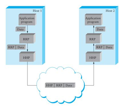
Figure 1.12 High-level messages are encapsulated inside of low-level messages.
