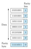
Figure 2.16 Two-dimensional parity.
