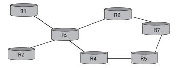
Figure 4.44 A network requiring explicit routing.
