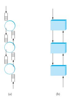
Figure 1.16 Alternative process models: (a) process-per-protocol; (b) process-per-message.
