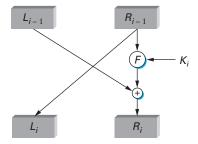
Figure 8.5 Manipulation at each round of DES.
