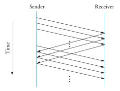
Figure 2.21 Timeline for the sliding window algorithm.
