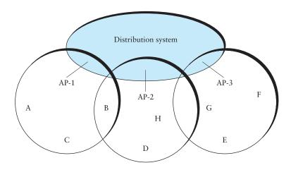
Figure 2.39 Access points connected to a distribution network.
