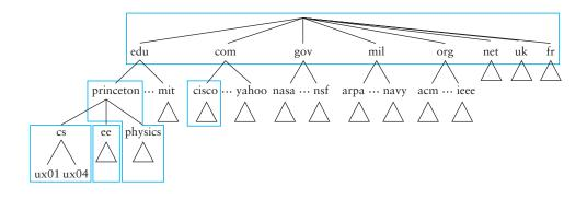
Figure 9.3 Domain hierarchy partitioned into zones.
