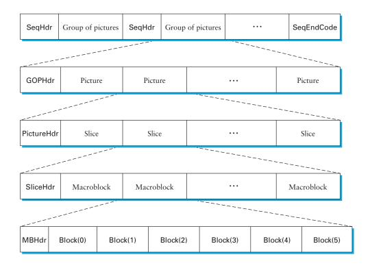
Figure 7.15 Format of an MPEG-compressed video stream.
