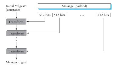
Figure 8.8 Overview of message digest operation.
