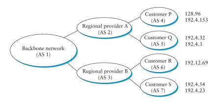
Figure 4.30 Example of a network running BGP.
