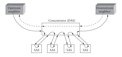
Figure 2.35 SASs connected to a concentrator.
