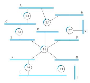
Figure 3.12 Extended LAN with loops.
