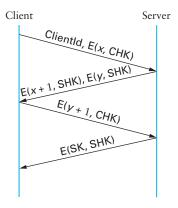
Figure 8.9 Three-way handshake protocol for authentication.
