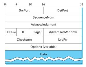
Figure 5.4 TCP header format.
