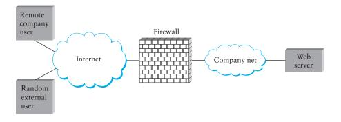
Figure 8.21 Firewall protecting a company Web server from some external accesses.
