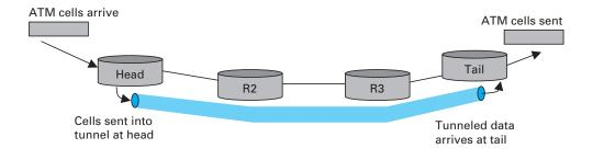
Figure 4.45 An ATM circuit is emulated by a tunnel.
