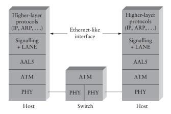
Figure 3.25 Protocol layers in LAN emulation.
