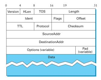
Figure 4.3 IPv4 packet header.
