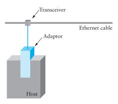
Figure 2.24 Ethernet transceiver and adaptor.
