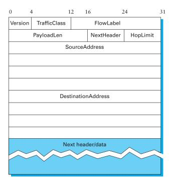
Figure 4.34 IPv6 packet header.
