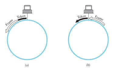
Figure 2.32 Token release: (a) early versus (b) delayed.
