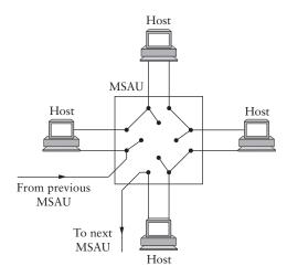
Figure 2.31 Multistation access unit.
