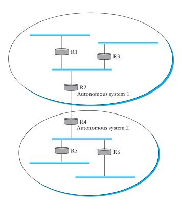
Figure 4.28 A network with two autonomous systems.
