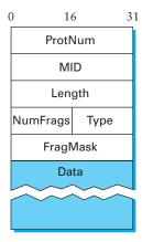
Figure 5.14 Format for BLAST message header.
