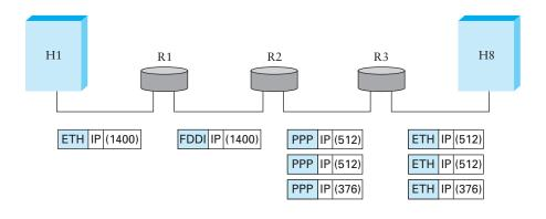
Figure 4.4 IP datagrams traversing the sequence of physical networks graphed in Figure 4.1.
