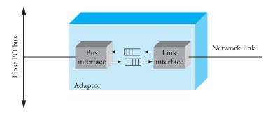
Figure 2.42 Block diagram of a typical network adaptor.
