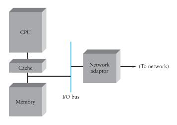
Figure 2.1 Example workstation architecture.
