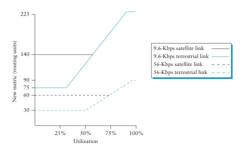
Figure 4.22 Revised ARPANET routing metric versus link utilization.
