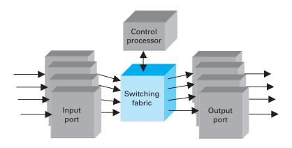
Figure 4.7 Block diagram of a router.
