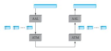
Figure 3.17 Segmentation and reassembly in ATM.
