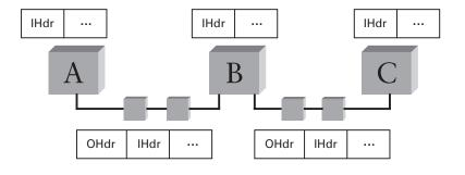
Figure 9.18 Overlay nodes tunnel through physical nodes.
