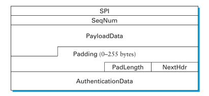
Figure 8.19 IPSEC's ESP header.
