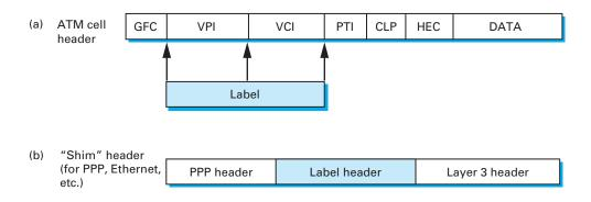
Figure 4.42 (a) Label on an ATM-encapsulated packet. (b) Label on a frame-encapsulated packet.
