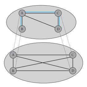
Figure 9.20 Multicast tree embedded in an overlay mesh.
