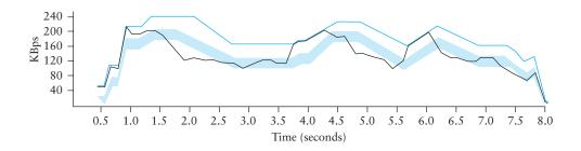
Figure 6.19 Trace of TCP Vegas congestion-avoidance mechanism. Top, congestion window; bottom, expected (colored line) and actual (black line) throughput. The shaded area is the region between the  $\alpha$  and  $\beta$  thresholds.
