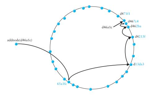
Figure 9.26 Adding a node to the network.
