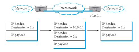
Figure 4.13 A tunnel through an internetwork.
