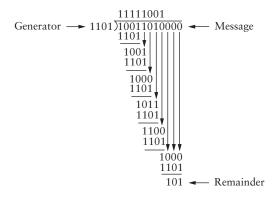
Figure 2.17 CRC calculation using polynomial long division.
