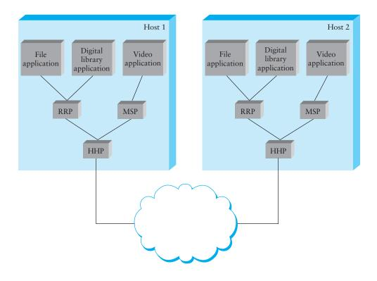
Figure 1.11 Example of a protocol graph.
