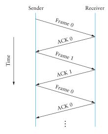
Figure 2.20 Timeline for stop-and-wait with 1-bit sequence number.
