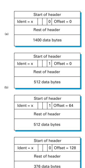
Figure 4.5 Header fields used in IP fragmentation. (a) Unfragmented packet; (b) fragmented packets.
