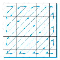
Figure 7.12 Zigzag traversal of quantized frequency coefficients.
