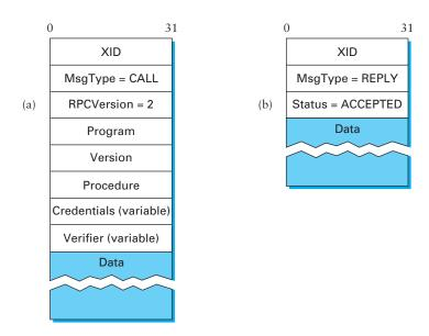
Figure 5.20 SunRPC header formats: (a) request; (b) reply.
