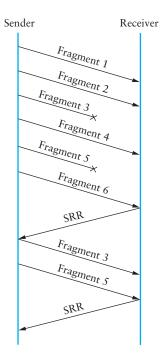
Figure 5.13 Representative timeline for BLAST.
