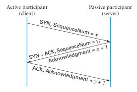
Figure 5.6 Timeline for three-way handshake algorithm.
