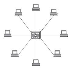
Figure 3.1 A switch provides a star topology.
