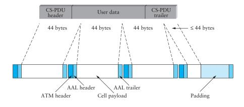
Figure 3.20 Encapsulation and segmentation for AAL3/4.
