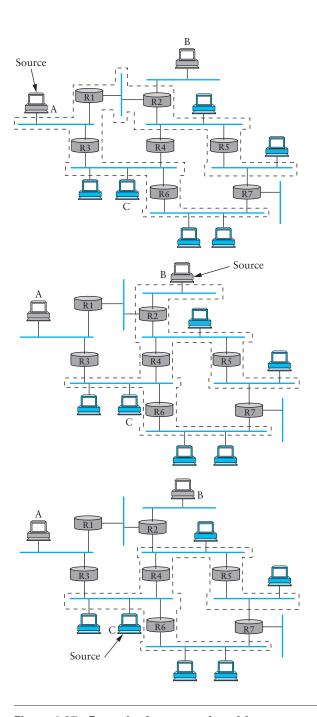
Figure 4.37 Example shortest-path multicast trees.
