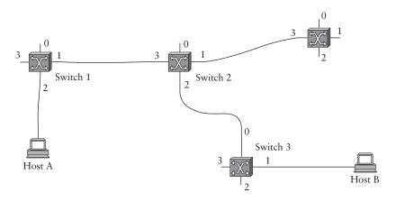
Figure 3.5 An example of a virtual circuit network.
