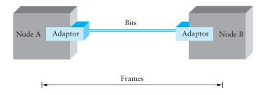
Figure 2.8 Bits flow between adaptors, frames between hosts.
