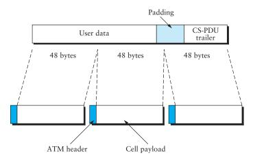
Figure 3.22 Encapsulation and segmentation for AAL5.
