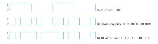
Figure 2.37 Example 4-bit chipping sequence.
