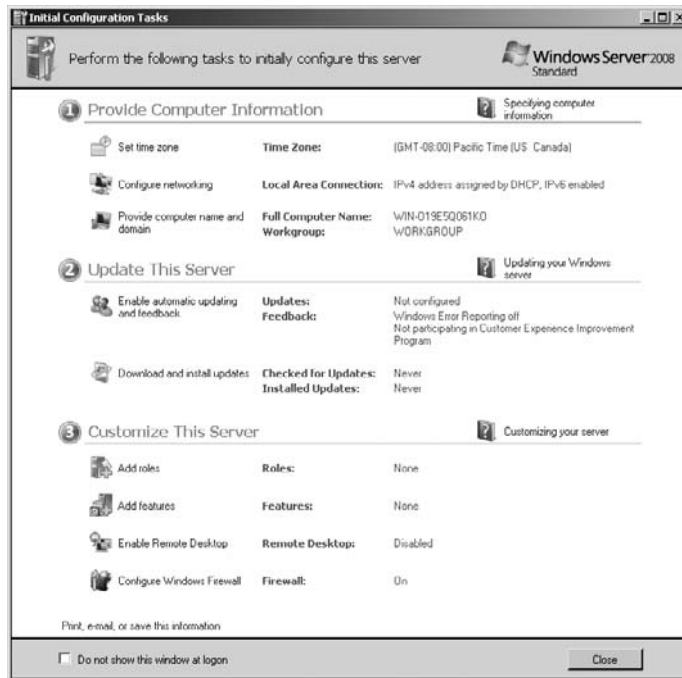
Figure 16-10. The Initial Configuration Tasks window appears after installation
