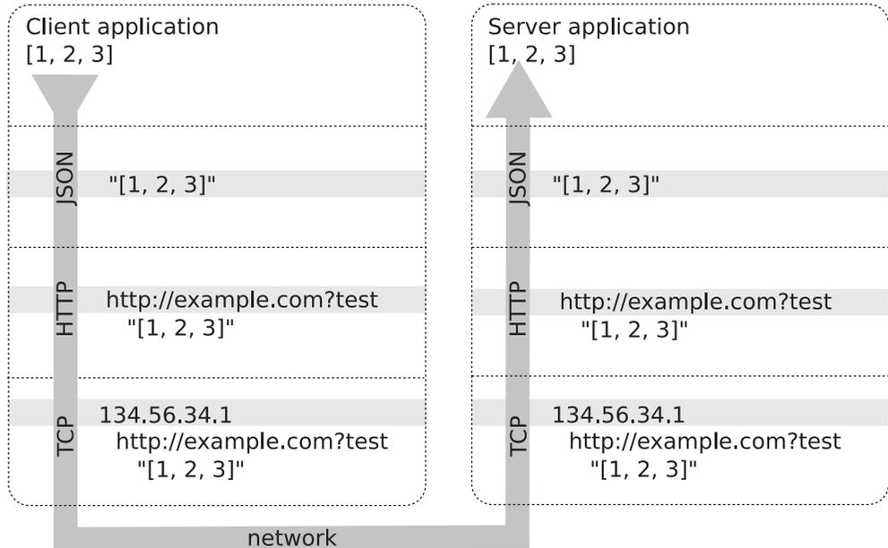
**Figure 8.3** Sending data from a client to a server using the full JSON/HTTP/TCP protocol stack
