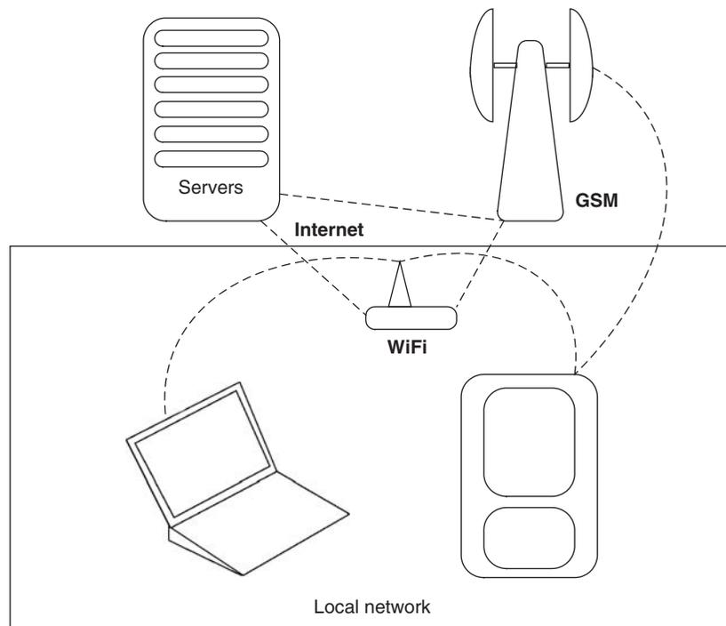
**Figure 8.1** Networking environment of a modern mobile phone
