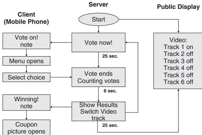
**Figure 11.1** State diagram of the MobiLenin system
