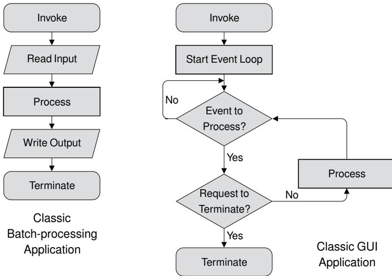
**Figure 4.2** *Batch processing applications versus GUI applications*
