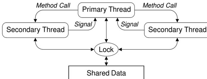
**Figure 19.2** A schematic of typical PyQt inter-thread communication
