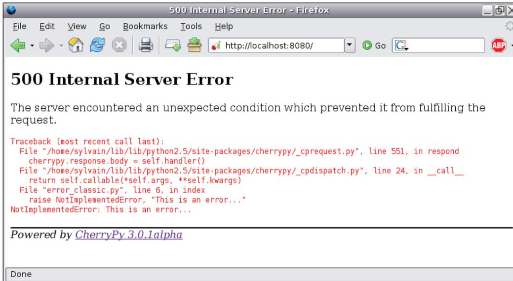
As you can see CherryPy displays the complete traceback of the Python error. Although this is useful when developing the application, it might not be relevant in production mode. In that case, CherryPy returns simply a default message.
