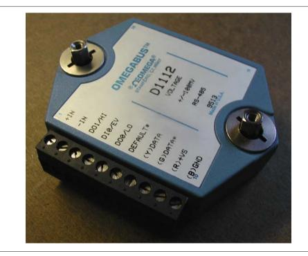
Figure 14-3. Omega D1112 RS-485 data transmitter
