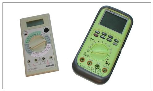
*Figure 6-3. Digital multimeters*
