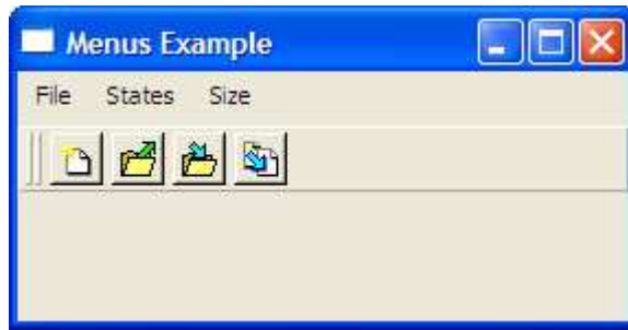
Figure 13.4: Use a toolbar for immediate access to commonly used commands.
