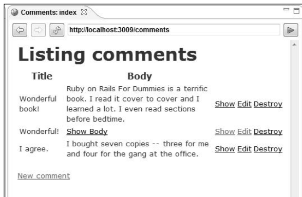
Figure 13-2: Comment bodies in place of some links.
