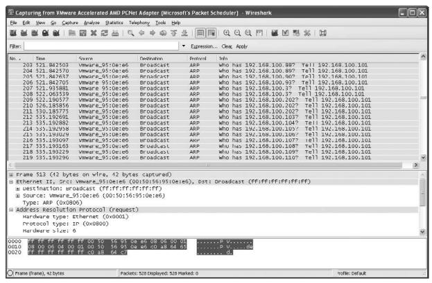
FIGURE 4-2 Traffic generated by Nmap scan
