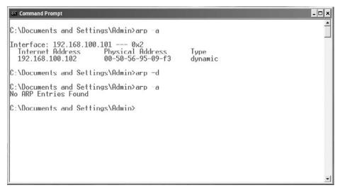
FIGURE 1-4 The arp command in Windows
