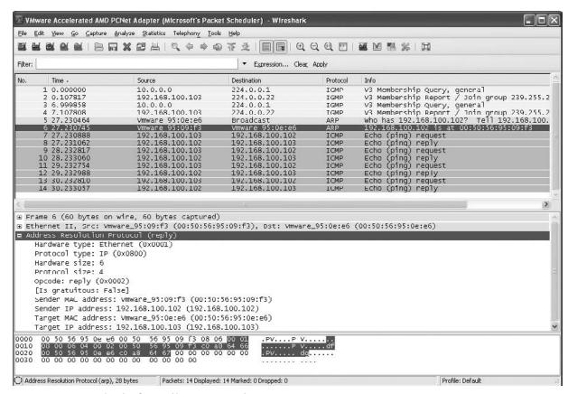
FIGURE 2-3 Wireshark after collecting ping data
