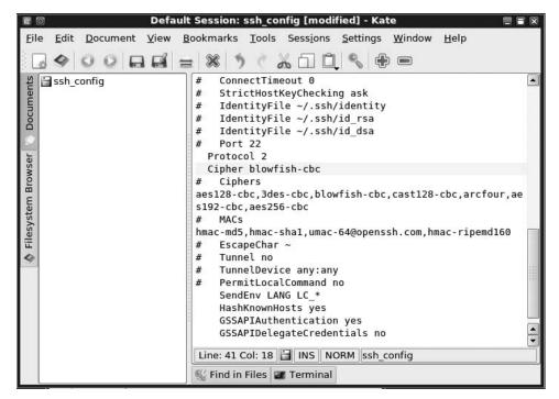
FIGURE 8-6 Configuring the SSH client in Linux
