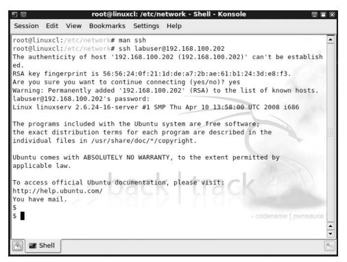
FIGURE 8-2 Connecting with SSH
