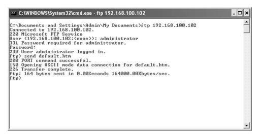
FIGURE 3-1 Uploading a web page with the ftp command in Windows
