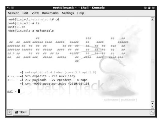
FIGURE 4-4 The Metasploit console
