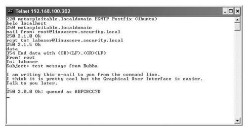
FIGURE 3-4 Using Telnet and SMTP to send an e-mail
