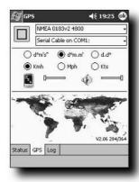
FIGURE 7-11: Pocket PC software is similar to most desktop PC software in that it will have port settings information.
