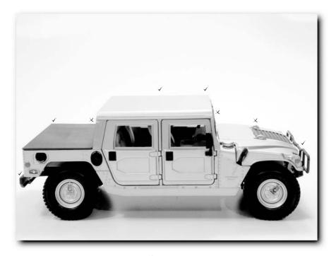
FIGURE 4-10: Good and bad placements for antenna on a car
