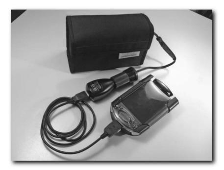
FIGURE 11-23: Portable lead-acid battery
