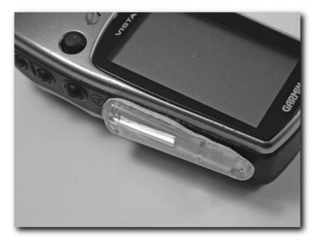
FIGURE 11-32: Attaching the Glowring
