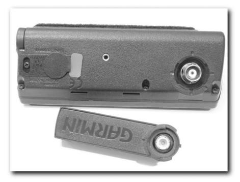
FIGURE 4-6: A Garmin III GPS receiver with the antenna removed
