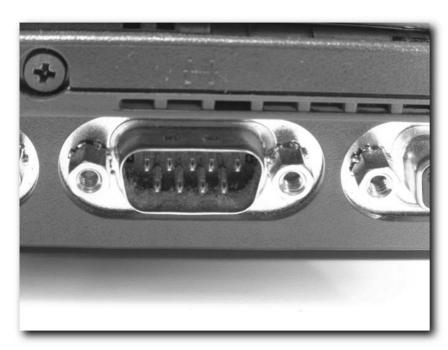
FIGURE 7-4: A PC serial port
