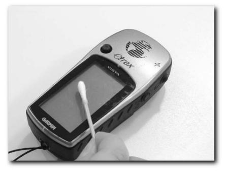
FIGURE 5-3: Carefully clean the screen before applying the screen protector.
