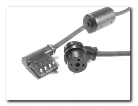
FIGURE 2-3: Two GPS connectors
