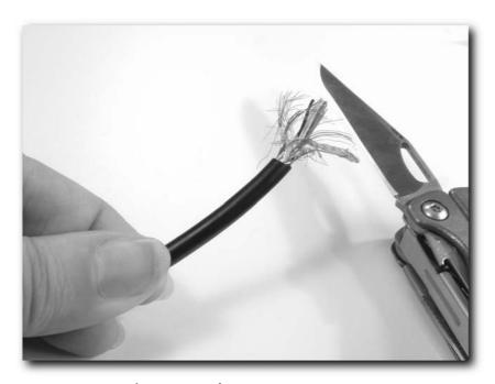
FIGURE 2-5: Exposing the inner core of wires
