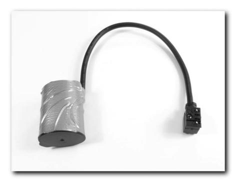
FIGURE 3-19: Completed film pot battery holder
