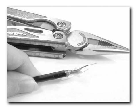
FIGURE 2-8: Trimming back the sheathing
