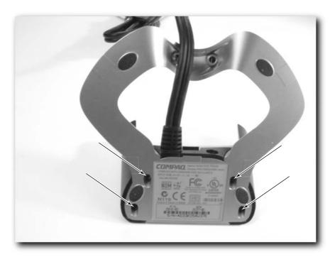
FIGURE 2-25: You need to undo these screws.
