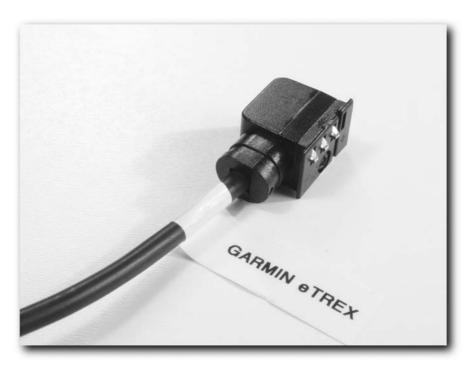
FIGURE 2-23: Label cables clearly to avoid confusion.
