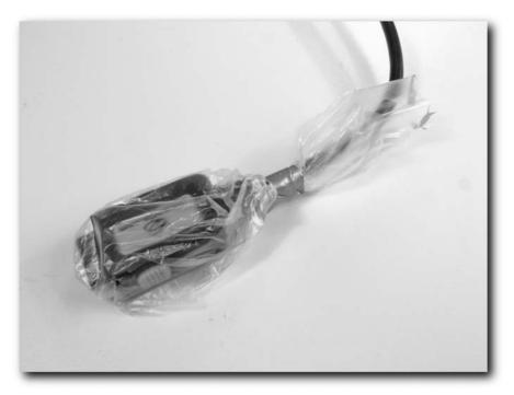
FIGURE 11-18: Connector protected by a small plastic bag
