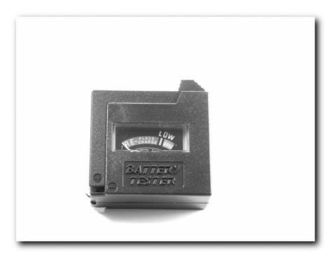
FIGURE 11-24: Battery tester
