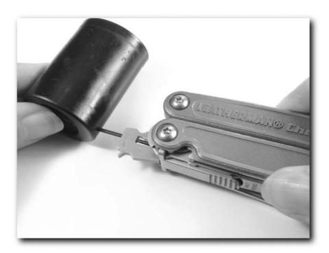
FIGURE 3-14: Carefully make a hole in the bottom
