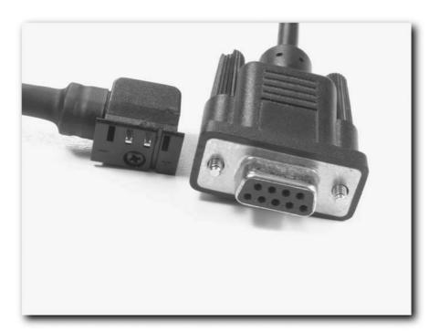
FIGURE 2-1: A PC-to-Garmin eTrex data cable
