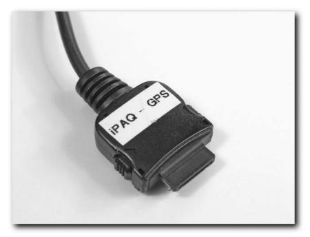
FIGURE 11-17: Clearly labeled cables
