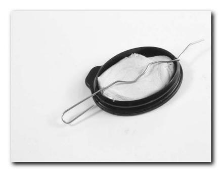
$\label{figure 3-17} \textbf{Figure 3-17: The top of the completed film pot. Note the notches at either end of the lid accommodating the wire for the terminals. }$
