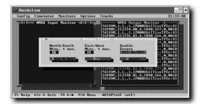
FIGURE 9-11: Adding errors to the simulated GPS data
