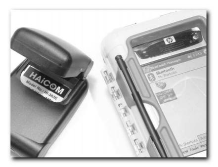
FIGURE 5-27: The flexible plastic film on the front enables you to use your device while it is still in the case.
