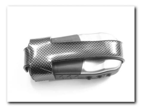
FIGURE 5-40: Mold the warm Concealex on the GPS.
