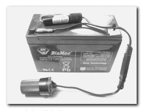
FIGURE 3-5: A fused 12-volt lead-acid battery
