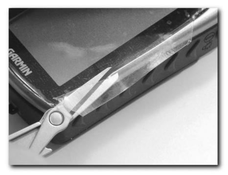
FIGURE 5-7: Carefully cut around the edges of the screen protector.
