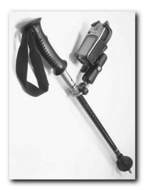
FIGURE 5-34: Bike mount attached to a ski pole
