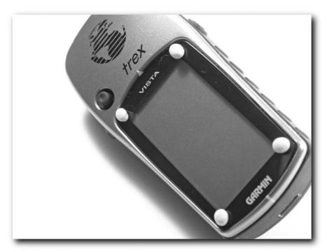
FIGURE 11-33: Rubber bumpers add simple screen protection.
