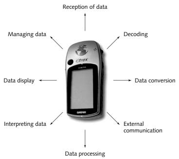
FIGURE 6-1: The basic functions of a GPS receiver
