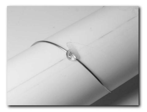
FIGURE 4-19: Partly completed helix coil
