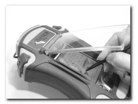
FIGURE 5-28: The well-armored Otter 3600 has a flip-down polycarbonate covering to shield the plastic film on the front.
