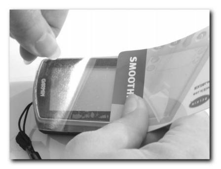
FIGURE 5-6: Using the plastic card to work out bubbles in the plastic film is vital.
