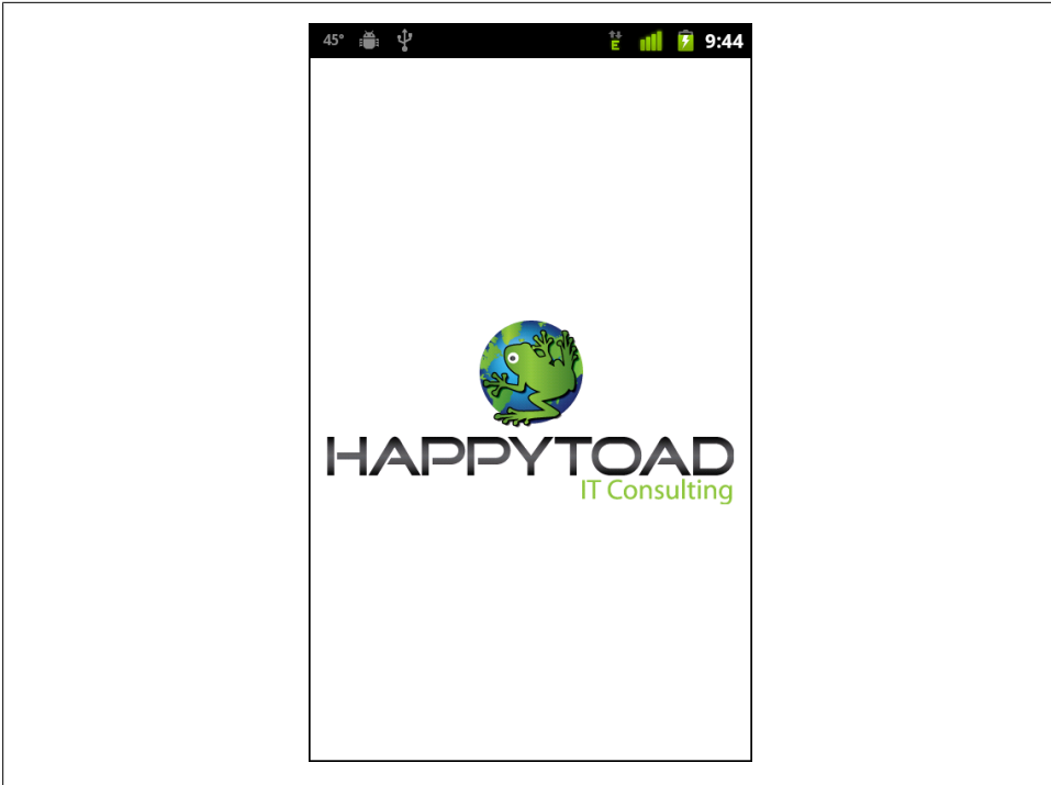
Figure 6-10. Splash screen with splashScreenScaleMode set to none
