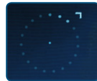
EXAMPLE OF A GIMBALED WEAPON NOT YET PROPERLY ALIGNED TO THE LOS MARKER
