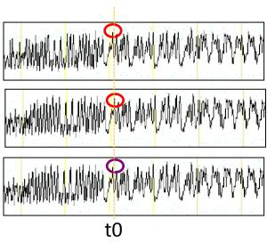
Distribution of signal amplitude where register 7 bit 1 = 0 is different from distribution where register 7 bit 1 = 1
