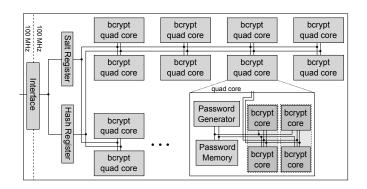
Figure 1. Schematic Top-Level view of FPGA implementation. The design uses multiple clock-domains: a (slow) interface clock and a fast bcrypt clock. Each quad-core accesses the salt- and hash registers and consists of a dedicated password memory, four bcrypt cores and a password generator.
