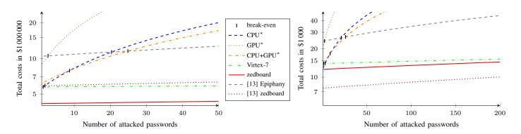
Figure 5. Total costs in *millions USD* for attacking n passwords of length 8 from a set of 62 characters, with logarithmic scale. Each attack finishes within *one month*. Both the acquisition costs for enough devices and the total power costs where considered.
