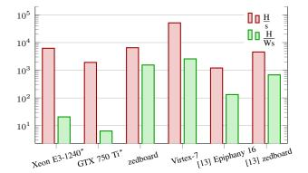
Figure 4. Comparison of different implementations for cost parameter 5. Left bars (red) show the hashes-per-seconds rate, right bars (green) the hashes-per-watt-seconds rate. Results with \* were measured with (ocl)Hashcat. The axial scale is logarithmic.
