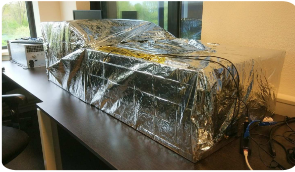
Shielded box with emergency blankets
