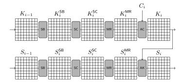
**Fig. 3.** One round of the block cipher W, used in the Whirlpool compression function.
