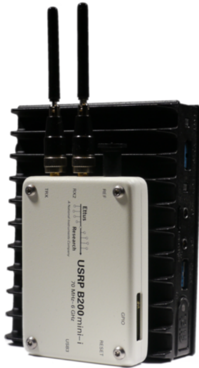
Fig. 7. Rogue Base Station USRP B200-Mini with a Fitlet2
