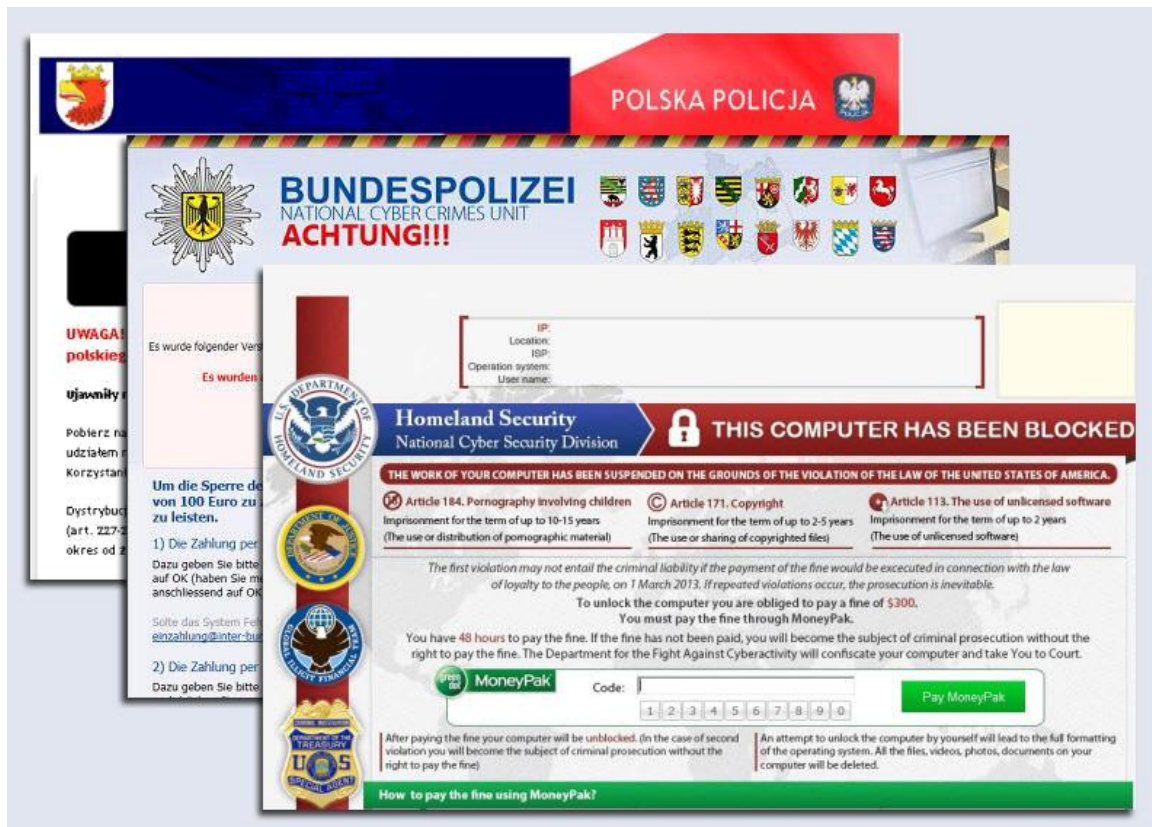
Figure 44. Examples of the lock screens used by different ransomware families, masquerading as warnings from various national or regional police forces
