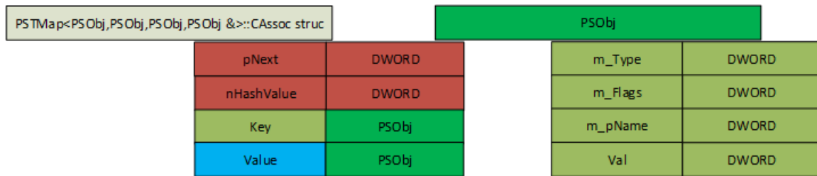
Figure 17. Memory layout of CAssoc structure and its embedded PSObjs
