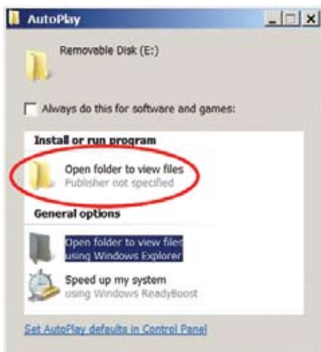
FIGURE 23. Win32/Conficker.B creates a fake AutoPlay option (circled) on removable disks; an unprotected user who chooses the wrong “Open folder to view files” option may become infected.
