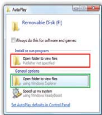
FIGURE 52. Worm:Win32/Conficker.B creates a fake AutoPlay option (in red) on removable disks. An unprotected user who chooses the wrong “Open folder to view files” option may become infected.
