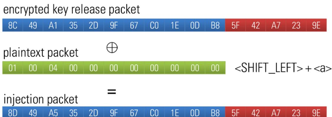
Figure 19: Example of keystroke injection
