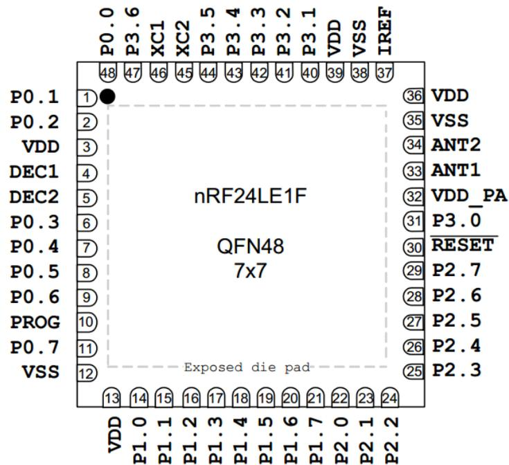
Figure 3: nRF24LE1F pin assignment for a QFN48 package [12]
