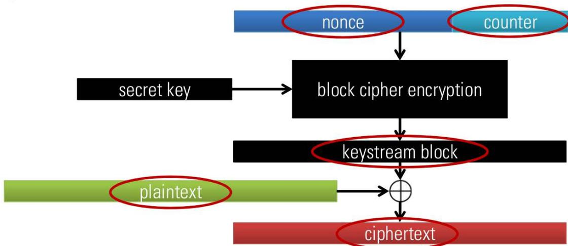
Figure 17: Counter mode encryption
