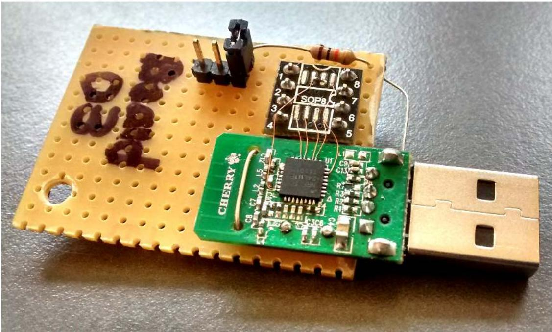
Figure 7: SPI read and write access to a Cherry USB dongle (thanks to Alexander StraÙheim)
