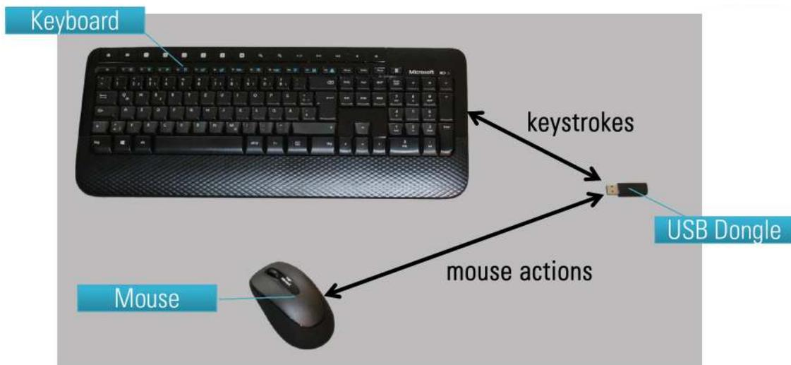
Figure 2: Simplified communication of wireless desktop sets
