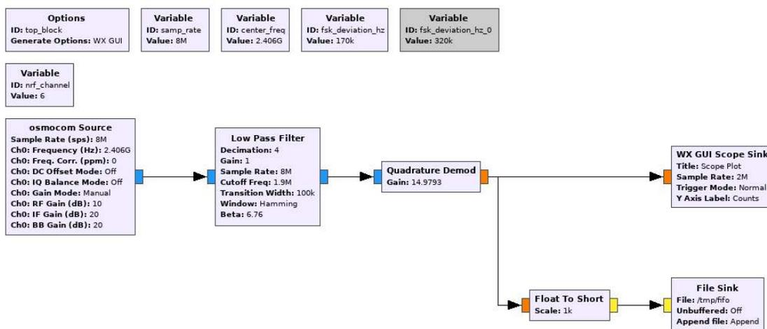
Figure 9: Simple GNU Radio Companion flow graph for use with modified version of NRF24-BTLE-Decoder
