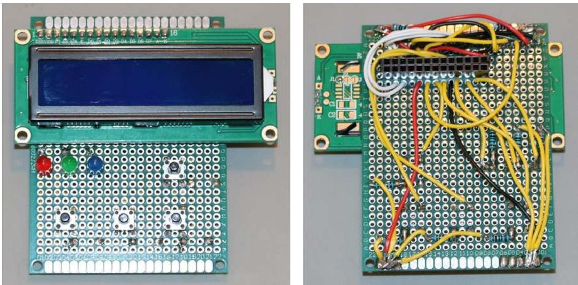
Figure 22: Very simple Raspberry Pi shield
