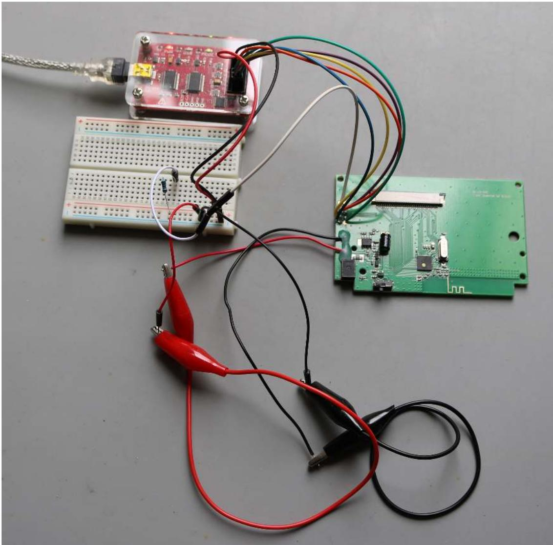
Figure 6: SPI read and write access to a Cherry wireless keyboard
