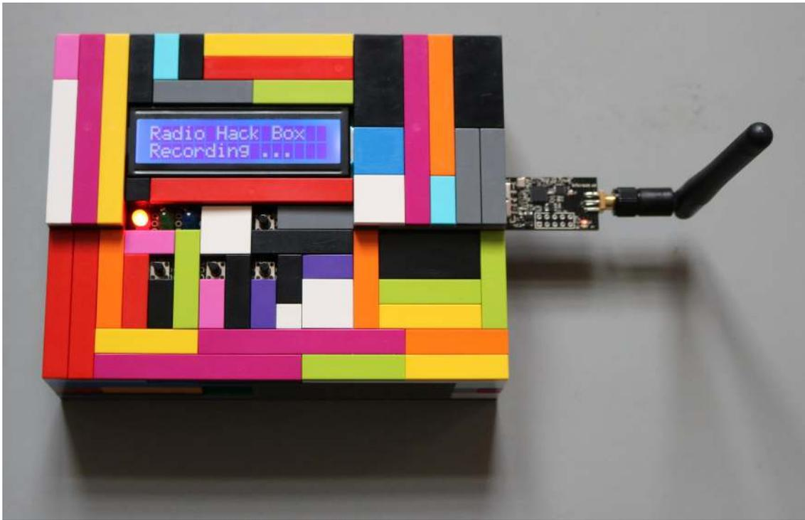
Figure 21: SySS Radio Hack Box prototype
